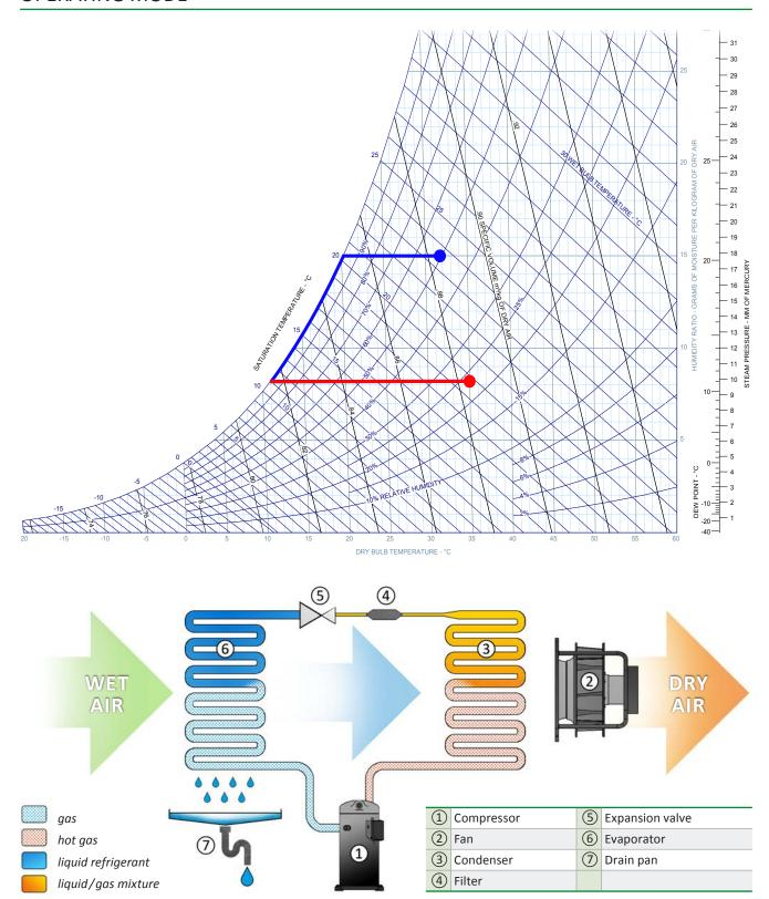
In practice, in a dehumidifier operating with a refrigeration cycle, the air passes through a finned evaporator, in which it is cooled by evaporation of the refrigerant gas; the dew temperature is reached and the water vapour condenses in the form of drops on the fins of the evaporator.
